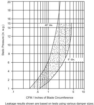
Leakage results shown are based on tests using various damper sizes. The shaded area between the graph lines indicate normal expected leakage range for a standard damper operating conditions and sizes.
